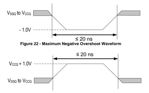
Figure 23 - Maximum Positive Overshoot Waveform
