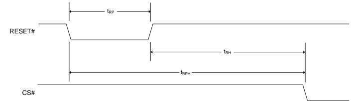
Figure 21 - Hardware Reset Timing Diagram
