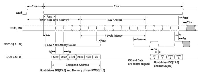
Figure 30 - Write Timing Diagram — No Additional Latency
