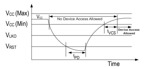
Figure 20 - Power Down or Voltage Drop
