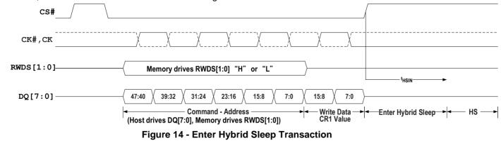
Note: DQ[15:8] input will be not used for command/Address decoding or as the write data, however, the controller has to drive DQ[15:8] to "H" or "L".
