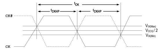
Figure 26 - Clock Characteristics
