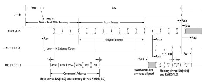
Figure 27 - Read Timing Diagram — No Additional Latency Required
